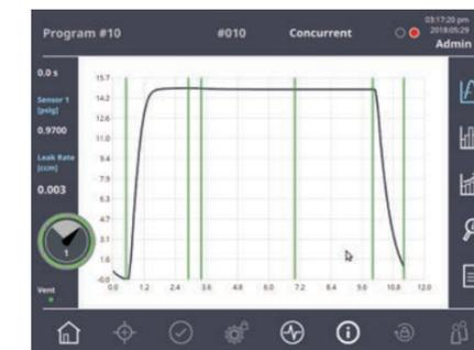
The reimagined touchscreen provides access to a wide range of data. From statistics like pass, fail, minimum, maximum, and standard deviations, to historical graphs and charts, the Sprint<sup>MD</sup> provides a deep level of information, making it easy to monitor the process.
