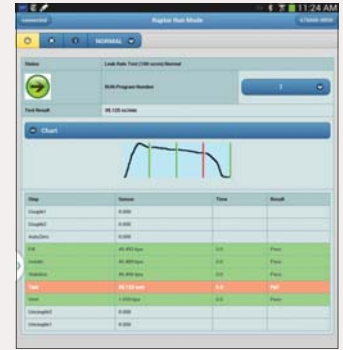
Completed "Fail" Test
